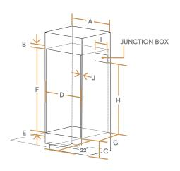
Allow a minimum of 22" for clearance to adjacent corners, drawers, walls, etc. when door is open.
