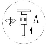
When adjusting the height of the steel wire, the telescopic metal part A toothed outer ring can only twist half a turn, and then pull it up to adjust the height!!!
