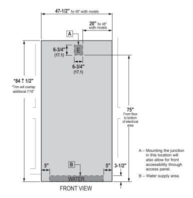
NOTE: GFI (ground fault interrupter) is not recommended. Water line can enter the opening through the floor or rear wall. The water line installed should be 1/4" O.D. copper tubing or GE SmartConnect™ tubing between the cold water line and water connection location. The line should be long enough to extend to the front of the refrigerator. Installation of an easily accessible shutoff valve in the water line is required.
