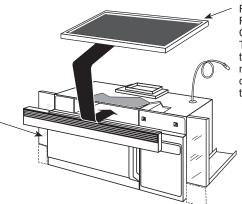
Filter Kit JX81L— Recirculating Charcoal Filter Kit To be used when the Spacemaker microwave oven cannot be vented to the outside.
