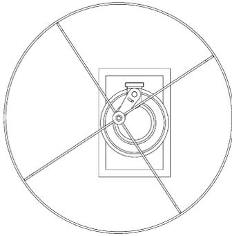
Position of diffuser plate to replace bulb.
