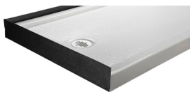
Factory-installed tile flange is 3/16" thick. Account for this thickness when planning final opening size.
