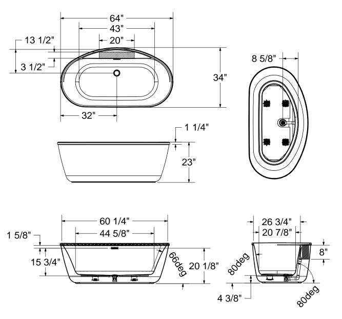
(() Recommended faucet area 1 section of 20" (L) x 3 1/2" (W). Depth recommended for straight pipes 8".
