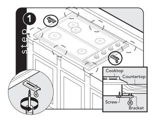
Screw hold down brackets to the burner box using the  $\#10 \times 1/2"$  sheet metal screws. There are 6 bracket assemblies included. There must be a minimum of 2 brackets installed with the possibility of up to 6 in locations noted depending on installation
