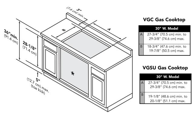
\*Note: Refer to the oven installation instructions for undercounter dimensions. Installation will require an elbow to be installed off of the regulator.
