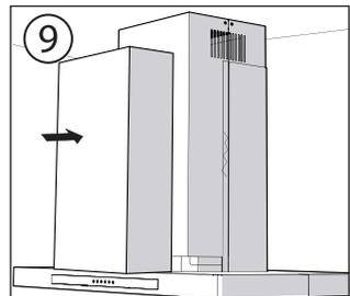
9. Verify that ducting from hood is connected to ducting in the attic that will exhaust air out of the home.
