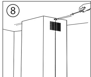
8. Secure the two lower duct covers to the support frame by overlapping the lateral magnets. Fig.9
